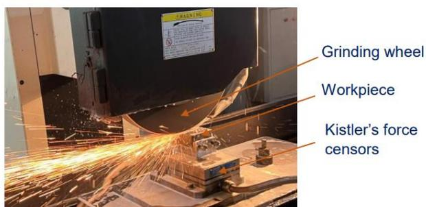
Fig. 1. Configuration for the experiment
