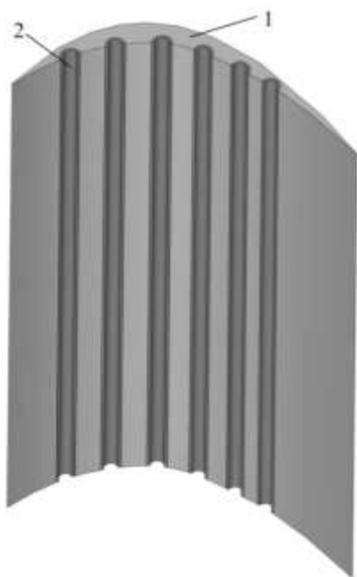
Figure 1. Turbine blade in section: 1 – turbine blade body, 2 – capsule
