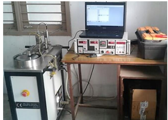
Fig. 2 Pin on disk experimental setup.
