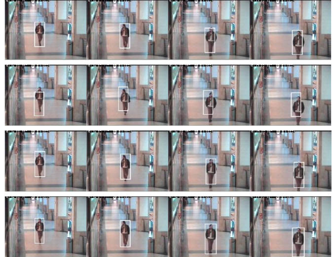
Fig. 9 Feature fusion and metric learning tracking results of pedestrian recognition sequence MAN in public environment
