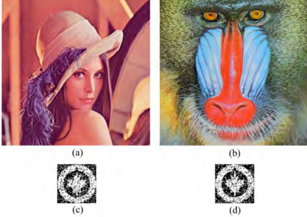
Fig. 9. An example of JPEG compression attack and watermark extraction with JPEG quality factor of 40: (a) compression of watermarked image of Lena at Fig. 7(b) with SNR=26.14 dB, (b) compression of watermarked image of Baboom at Fig. 7(d) with SNR=18.98 dB, (c) the extracted watermark from (a) with WAR=82.47 %, (d) the extracted watermark from (b) with WAR=83.42 %.
