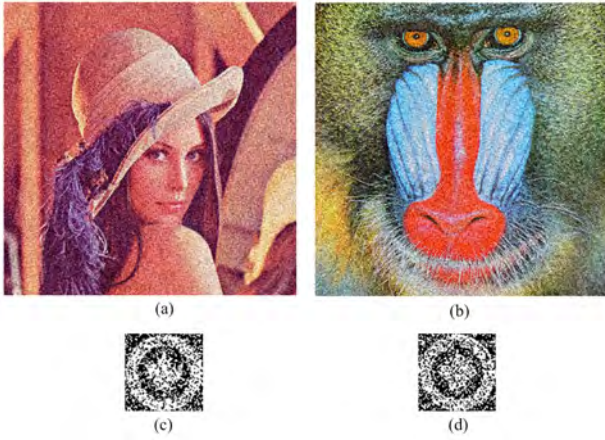
Fig. 13. An example of AWGN noise attack and watermark extraction with variance of AWGN= 40^2 : (a) attacked watermarked image of Lena at Fig. 7(b) with SNR= 10.9 dB, (b) attacked watermarked image of Baboom at Fig. 7(d) with SNR=10.74 dB, (c) the extracted watermark from (a) with WAR=75.34 %, (d) the extracted watermark from (b) with WAR=71.73 %.
