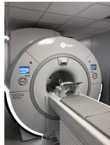
Fig. 1. The 3.0 T Signa Pioneer MRI scanner GE Healthcare
