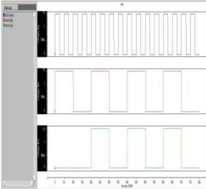
Fig 4.1(a): MOSFET based shift register output waveform at 90nm
