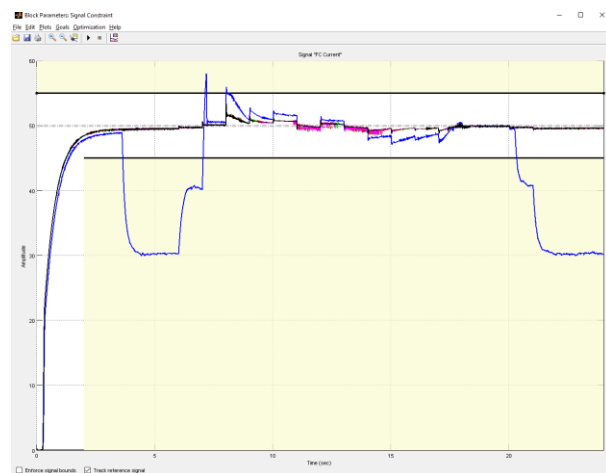
Figure 16. Graphical results of the optimization procedure for the capacitor of the second load profile with reference of the fuel cell 50A.
