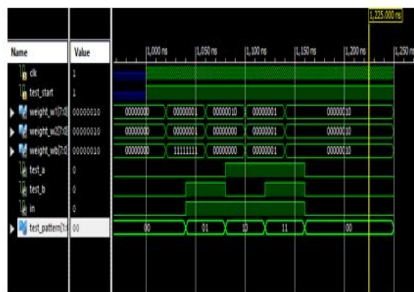
Fig. 4: Simulation results for weight generation using ISE Design Suite
