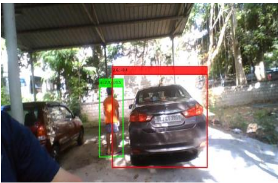
Figure 14 (a): The vehicle is closer to the ego vehicle than the threshold safe distance (5 meters)
