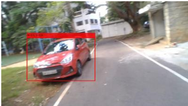
Figure 14 (b): The vehicle is closer to the ego vehicle than the threshold safe distance (4 meters)
