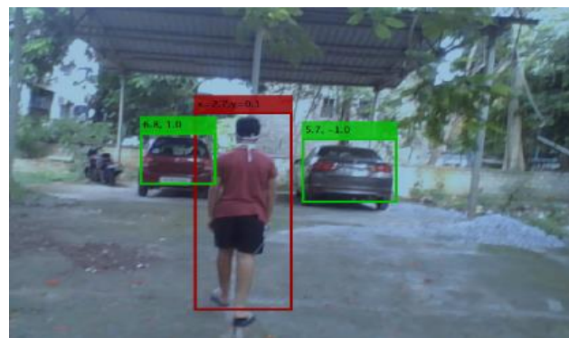
Figure 13 (a): The pedestrian, is closer to the ego vehicle than the threshold safe distance (3 meters)
