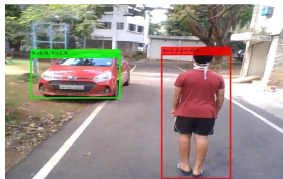
Figure 13 (b): The pedestrian, is closer to the ego vehicle than the threshold safe distance (3 meters)
