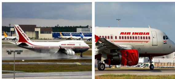
Fig.1 Thrust reversers deployed on turbofan of an Air India Boeing 747-400 landing at Indira Gandhi International Airport, New Delhi (left), Air India Airbus A319 with thrust reversers deployed on turbofan engine for pushback i.e. "Power Back" (right). [5]
