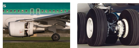
Fig. 2 Different decelerating devices installed on current commercial aircrafts including thrust reversers in turbofan engine (left) and wheel brakes in landing gears (right).
